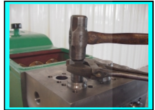
24. Use several firm to heavy blows with hammer to seat the valve after initial torque
