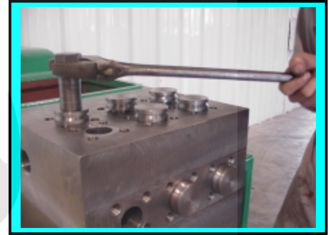
33. Re-torque valve retainer to 150 ft-lb
