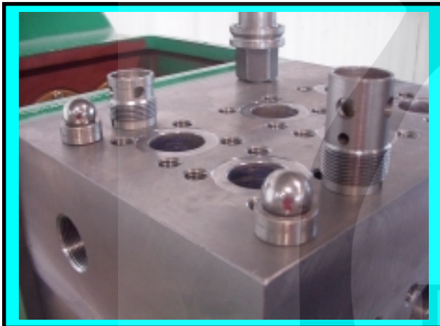
16. Suction and discharge valve retainer ball and seat shown
